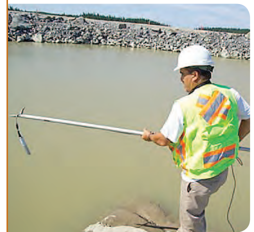
Water quality testing in isolated pond prior to discharging the water.
